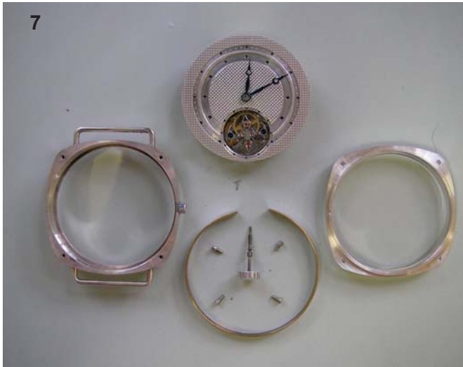
Figures 7 & 8 show the parts that make up two of the watches. I usually make the dial first as it forms part of the movement which has to be secured into the band of the case.
